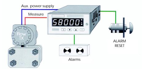
The DPL has a built-in 24 V auxiliary power supply able to supply 2-or 4-wire field transmitters.
