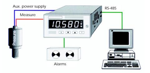
The DPL can be delivered with RS-485 optoisolated serial interface in order to allow the use of the instrument as a part of a computerized acquisition/ supervision system.
