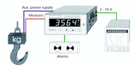
The DPL is available with an isolated analog retransmission which allows to solve a lot of plant problems like recording, trending or to display the measured value on field and in control room.
