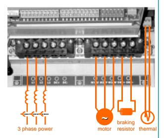
The power terminals shown are for frame D. Although other frames may vary slightly in appearance, their terminal designations and functionality are identical
