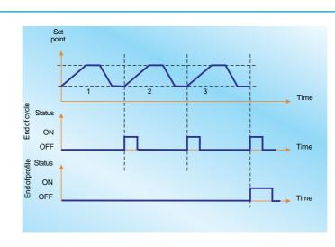
This example shows a program formed by 4 segments and it is repeated for 3 times.
